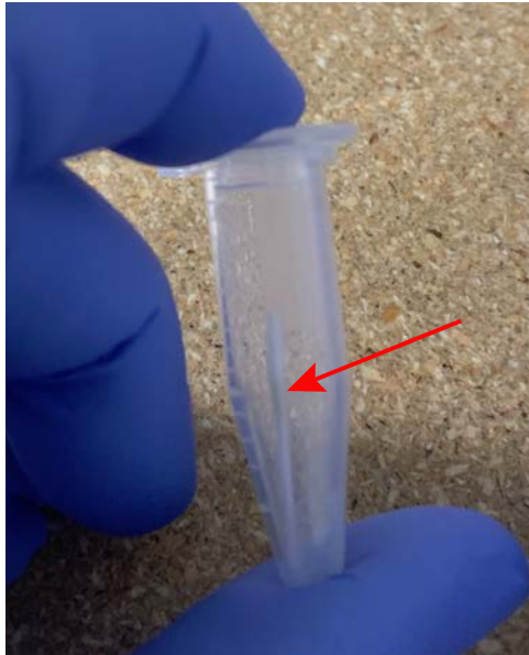
Figure 2- Representative image of a 5-10 \mu m FFPE Tissue scroll in a 1.7ml Microfuge Tube. The tip of the red arrow points to the FFPE section.
